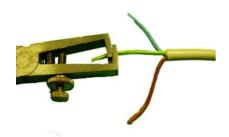
Use wire strippers to remove the insulation without damaging the conductors.
