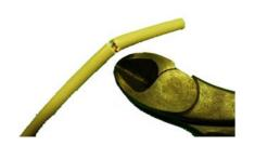
Cut away the outer sheath with a knife or a wire cutter, taking care not to damage the wires.
