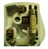
Loosen the three terminal screws.
