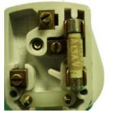
Loosen the terminal screws.
